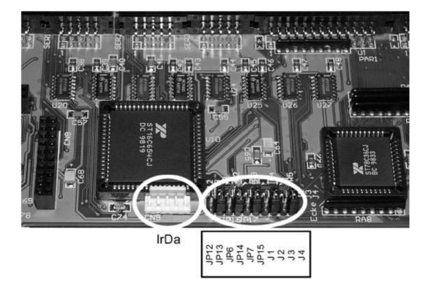
The Jumpers on the IOBlix are for special purposes only! The corresponding Jumpers are listed below. Important: Never set both of a pair of jumpers!
