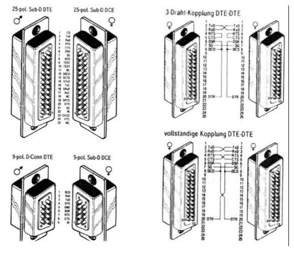
On the left hand side you see the pinning of the 9 and 25 pol connectors. On the right hand side you can see two different null modem connections where the "vollständige Kopplung DTE-DTE" should be preferred.
